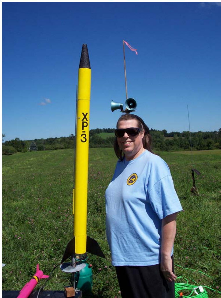
Photo: July 21, 2007 Syracuse Launch day, Cheryl Costa with her scratch built cluster rocket XP-3. (Airframe 3" commercial mailing tube)
